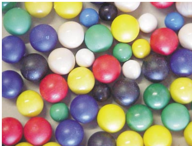
Figure 2. Mechanical model of spheres of different colors and sizes to visualize local configurations, that is, grain contacts by n starting grains, to obtain the diversity of product grains distributed within the bulk sample.
